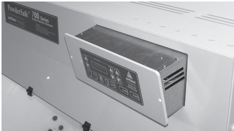
Figure 10, Removing the AirSafe™ controller from the AC730/AC740C model.
