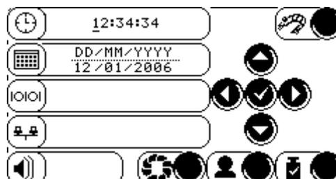
Using the arrows and the ok symbol all the parts of the screen can be changed
