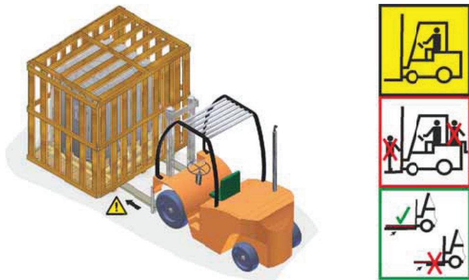
Fig. 9: Forklift prongs are pushed completely beneath the transport frame
