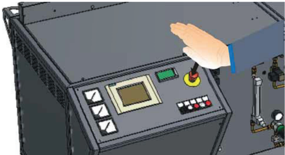
Fig. 8: Bringing the furnace to a stop in an emergency using the safety facility on the operating panel
