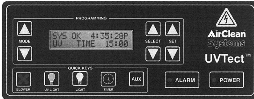
Figure 5, Control panel layout.
