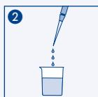
Fill 10 mL of sample into beaker (or cuvette)
