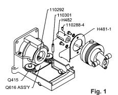
d) Tighten thumb NUTS and operate motor. If noisy, alter position of BRACK-ET under RETAINER PLATE slightly while operating until minimal noise position is found. Retighten thumb NUTS.
