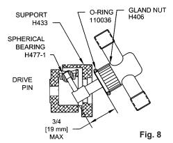
10 or 20 strokes at maximum setting, handling water (left to right mode facing pump head) with suction line blocked or pinched off. This will create a vacuum in the pump head, permitting atmospheric pressure to shape the outer seal member tightly around the piston.
