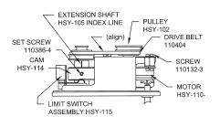
7. MOUNTING RH PUMP. For maximum pump performance, mount RH pump with motor at 12 O'Clock and pump head at 6 O'- Clock position. This orientation will allow air bubbles that enter the pumping chamber to directly exit through buoyant assist. Discharge lines should be inclined upward from pump head.
