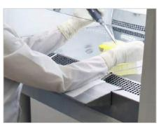
A removable armrest ensures reliable elbow support preventing operator's arms from hanging. Suitable for thorough disinfection and autoclave sterilization. Stored in a special compartment of the pullout UV unit.
