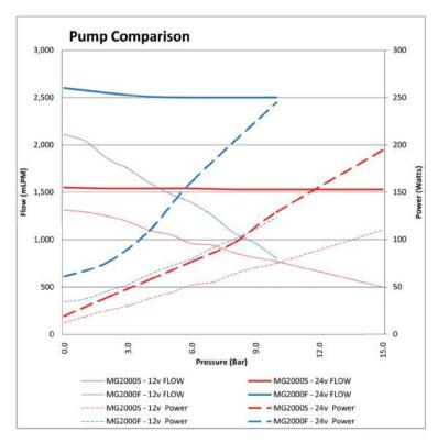
All tests conducted pumping TCS Coolant and using an EQi-MG2 motor controller. Note for maximium pump life you should not subject the MG2000S to pressures exceeding 10 bar and the MG2000F should not exceed 8 bar
