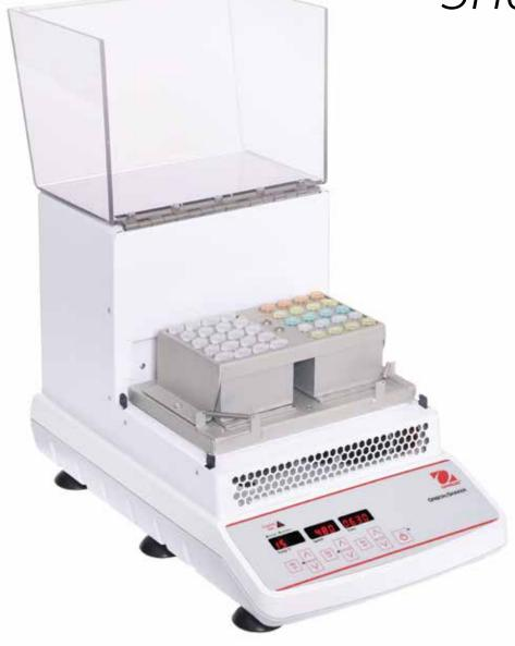
OHAUS Incubating Cooling Orbital Shakers are designed to incubate samples from 10° below ambient to 65°C. Incubating Cooling Mini Shaker is designed to hold two microplates or two optional modular tube blocks in a variety of configurations. All models feature touchpad controls with easy-to-read, independent LED displays for temperature, speed and time. Microprocessor control provides consistent uniform shaking action..
