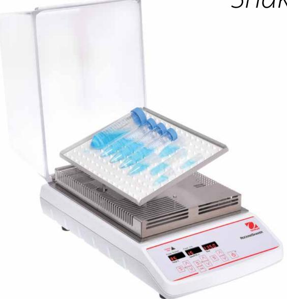
OHAUS Incubating Rocking and Waving Shakers are designed to incubate samples from 5° above ambient to 65°C to provide accurate and repeatable results. Rocking shakers provide a see-saw like motion, while waving shakers offer a smooth, low-foaming three-dimensional "wave" motion. All models feature LED displays with touchpad controls. Both models include safety features that protect both the user and samples.
