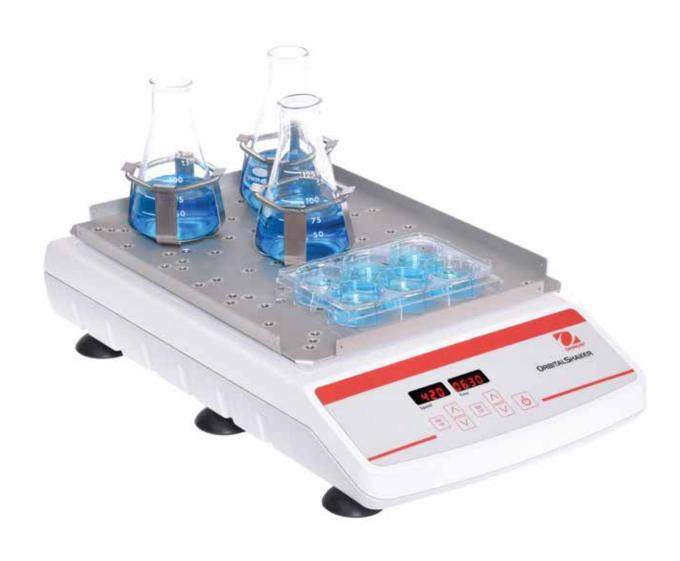
Light Duty Shakers are designed for applications with loads under 8 lb. Choose from two orbits and speed ranges to optimize your sample mix. Microprocessor-controlled and available as an analog model with basic speed control, two digital models which include a non-slip mat that can be removed to mount flask clamps and tube racks directly onto the tray, and a digital Microplate Shaker model which can hold up to 4 microplates or 2 microtube racks.
