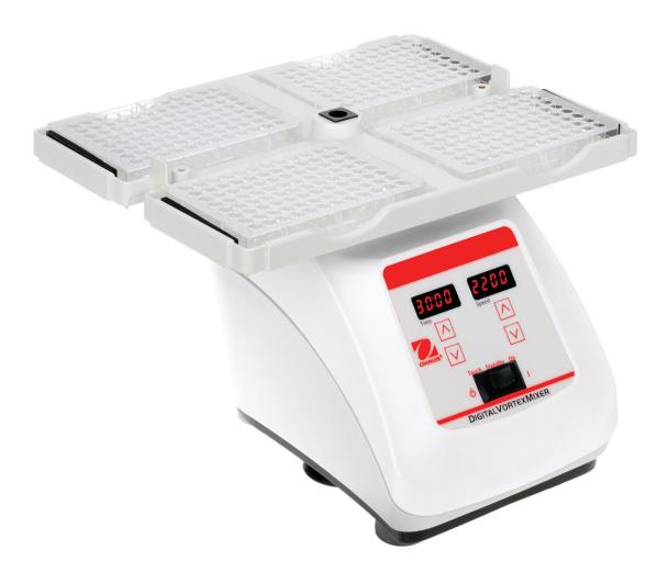
Heavy-Duty Vortex Mixers feature a heavy-duty design and efficient motor to permit continuous duty operation, and the ability to handle accessory components over the entire speed range. Analog variable speed models or microprocessor-controlled digital models offer exact speed control when applications demand repeatable results. A wide range of accessories are available for microtubes, microplates and a variety of tube sizes from 0.5 to 50 ml.
