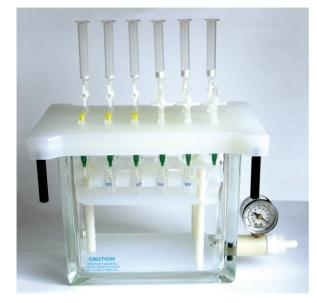
Teknokroma vacuum manifolds simplify SPE sample processing. These manifolds permit consistent extraction and filtration results. Analyst can save time, since these manifolds allow simultaneous multiple sample processing.
