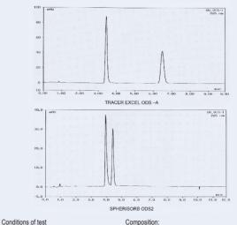
Eluant : Acetonitrile/Water, 30/70 1ml/min Lambda: 265nm
