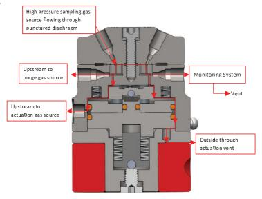
\* Complete isolation of process side from actuation/surrounding environment Ideal for unstable/reactive/toxic gas sampling applications
