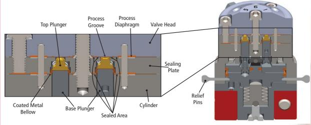
Isolation of the actuation by a coated metal diaphragm
