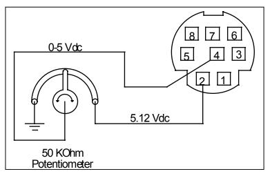
Simple method for providing set-point to controllers
