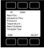
Press **DEVICE UNITS** to access menus of units of measure for each parameter (and totalizer if so equipped). Scroll to the desired unit and press select. Once selected, you will see the message shown below. Verify that all connected devices expect the change. See pages 49 and 50 for a full list of available units.
