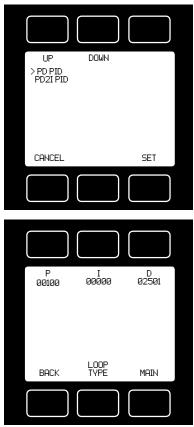
PID Values determine the performance and operation of your proportional control valve. These terms dictate control speed, control stability, overshoot and oscillation. All units leave the factory with a generic tuning designed to handle most applications. If you encounter issues with valve stability, oscillation or speed, fine tuning these parameters may resolve the problem.
