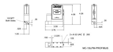
PROFIBUS MC1SLPM shown to provide PROFIBUS connector dimensions only. Flow body and valve dimensions will vary with range. Please see Alicat's device specifications for complete dimensions.
