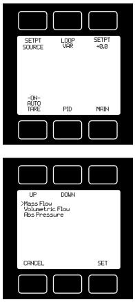
**LOOP VAR**—The selection of what variable to close the loop on is a feature unique to Alicat mass flow controllers.
