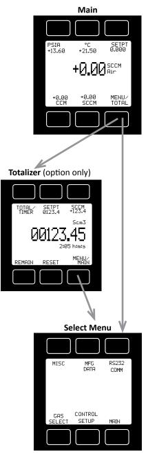
The **Main** display shows pressure, temperature, set-point, volumetric flow and mass flow.
