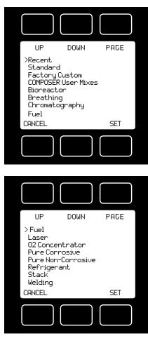
**Gas Select** allows you to set your device to up to 150 standard gases and mixes. You can also use **COMPOSER** to program and store up to 20 additional gas mixes.
