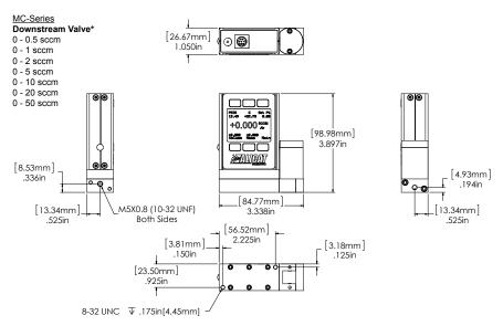
\* Note process connection port locations for downstream valve in this flow range.
