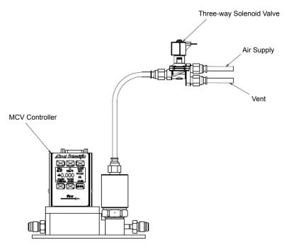
MCV controller and three-way solenoid valve.
