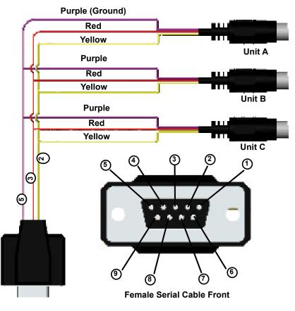
Typical Multiple Device (Addressable) Wiring Configuration
