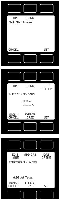
**Composer** allows you to program and save up to 20 custom gas mixes containing 2 to 5 component gases found in the gas lists (pages 40-47). The minimum resolution is 0.01%.
