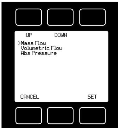
**LOOP VAR**—The selection of what variable to close the loop on is a feature unique to Alicat mass flow controllers.
