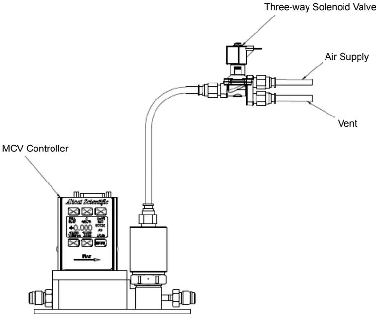
MCV controller and three-way solenoid valve.
