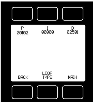
PID Values determine the performance and operation of your proportional control valve. These terms dictate control speed, control stability, overshoot and oscillation. All units leave the factory with a generic tuning designed to handle most applications. If you encounter issues with valve stability, oscillation or speed, fine tuning these parameters may resolve the problem.
