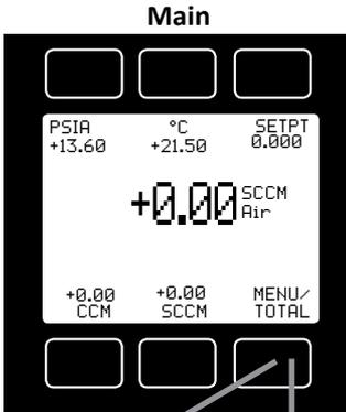
The **Main** display shows pressure, temperature, set-point, volumetric flow and mass flow.
