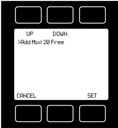
**Composer** allows you to program and save up to 20 custom gas mixes containing 2 to 5 component gases found in the gas lists (pages 40-47). The minimum resolution is 0.01%.
