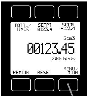
If your controller was ordered with the **Totalizer** option (page 54), pushing the **TOTAL** button once will bring up the **Totalizing Mode** display. Pushing **MENU** will bring up the **Select Menu** display.
