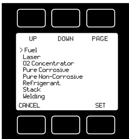
**Gas Select** allows you to set your device to up to 150 standard gases and mixes. You can also use **COMPOSER** to program and store up to 20 additional gas mixes.
