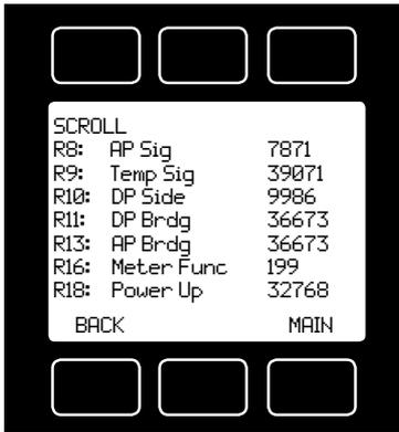
**DIAG TEST:** This diagnostic screen displays the current internal register values, which is useful for noting factory settings prior to making any changes. It is also helpful for troubleshooting with Alicat customer service personnel.
