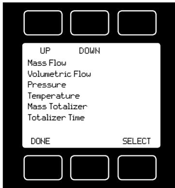
Press **DEVICE UNITS** to access menus of units of measure for each parameter (and totalizer if so equipped).
