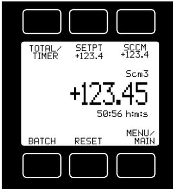
**TOTAL/TIMER:** Pushing the TOTAL/TIMER button will cycle the large numbers on the display between total mass and time elapsed.
