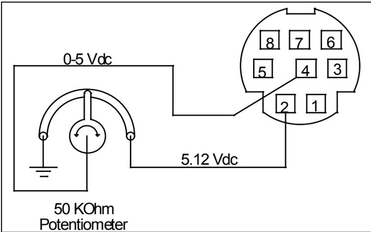
Simple method for providing set-point to controllers
