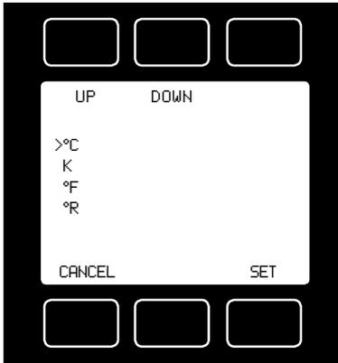
**Gas Temperature:** MC-Series flow controllers measure the incoming temperature of the gas flow. The temperature is displayed in degrees Celsius (°C). This parameter is moved to the primary display by pushing the button above °C.
