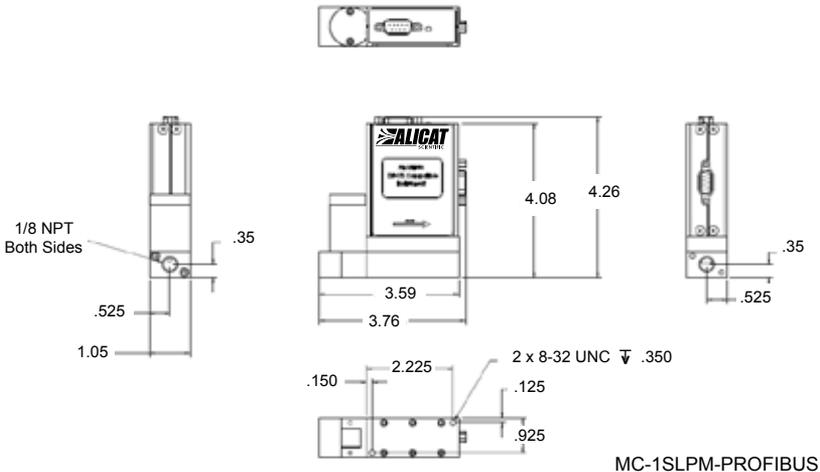
PROFIBUS MC1SLPM shown to provide PROFIBUS connector dimensions only. Flow body and valve dimensions will vary with range. Please see Alicat's device specifications for complete dimensions.
