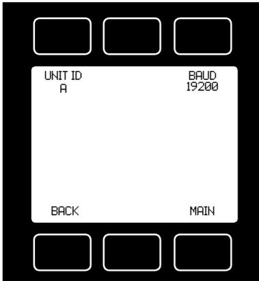
Access **Communication Select** by pressing the button above **RS232 COMM** or **RS485 COMM** on the **Select Menu** display.
