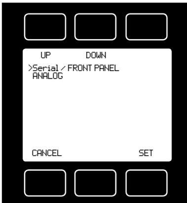
**Serial** refers to a remote digital RS-232 / RS-485 set-point applied via a serial connection to a computer or PLC as described in the installation and RS-232 / RS-485 sections of this manual.
