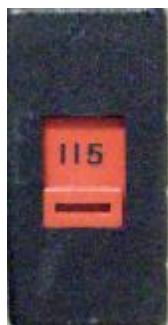
Voltage Selector Switch Set to 115V
