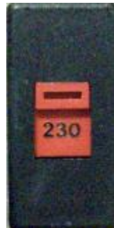
Voltage Selector Switch Set to 230V
