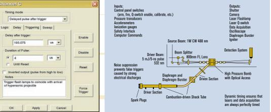
Trigger timing modes can be programmed via dialog controls. Logic is programmed using C-style syntax.
