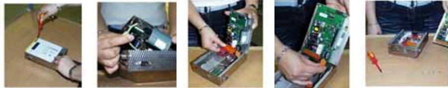
Fig. 28: Replacing a controller
