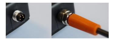
2. Connect the male part of the cable to the female connector on your instrument.
