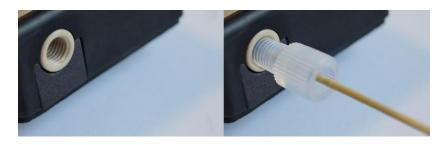
b) For a flow sensor with UNF 6-40 connectors first screw the UNF 6-40 - 1/4-28 adapter to the flow sensor, then screw the flangeless nut to the adapter.
