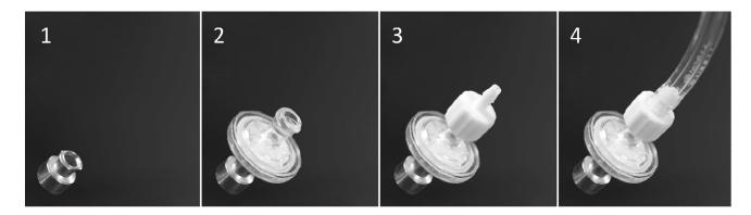
**Note:** the use of filters is highly recommended in order to prevent accidental insertion of liquids in the instrument due to backflow and generally does not affect performance. In some cases, however, it may increase settling time, especially when using large reservoirs (~100 ml). The removal of the filter – although not recommended - will render the instrument more responsive in this case.
