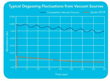
Fluctuations in detector baseline of a single-speed pump compared to the patented technology of the Systec ZHCR vacuum pump.\*
