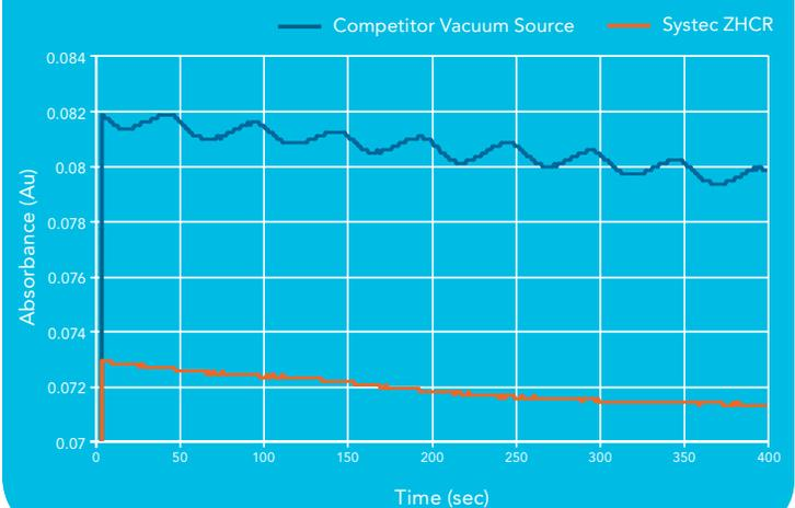
Fluctuations in detector baseline of a single-speed pump compared to the patented technology of the Systemc ZHCR vacuum pump.\*
