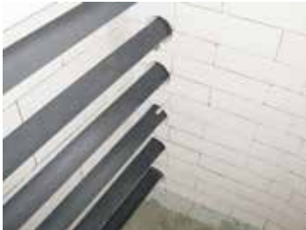
Heated on both sides by high performance SiC rods
