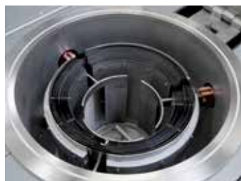
Cylindrical retort with tungsten heating
