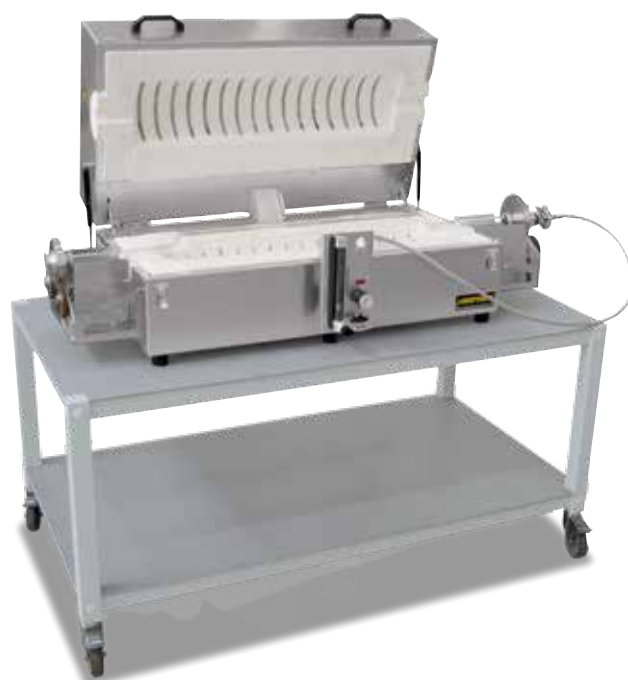
RSR-B 120/750/11 as tabletop version for batch operation
