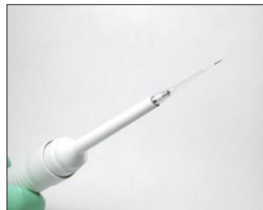
Figure 2 Trap'nTip™ fitted onto 10 µL pipette
