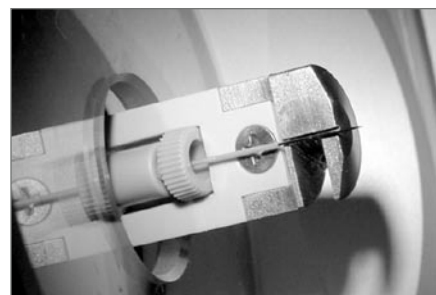
FIGURE 1 MicroTight® union holding a standard-length PicoTip® emitter
