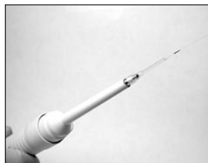
Figure 2 Trap'nTip™ fitted onto 10 µL pipette
