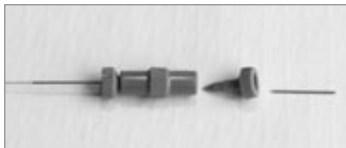
Figure 4 Union, compression fitting, and MicroTight® sleeve cut to 14 mm
