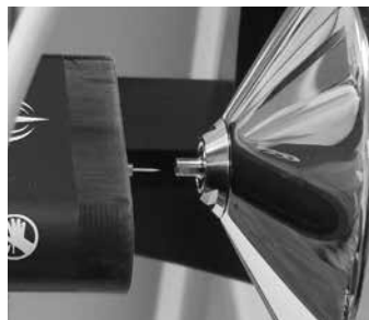
Figure 8: Push in activation button until it locks in place to engage voltage and expose emitter for spraying
