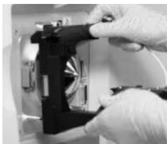
Figure 3: Installing the PicoChip source onto the instrument
