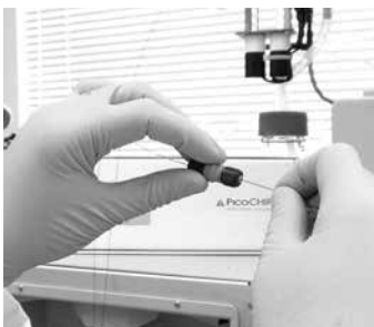
Figure 7: Connecting PicoChip pigtail to LC transfer line using an in-line filter (Upchurch p/n: M-538)
