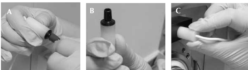
Figure 5: A) Remove the cover from the high-voltage cable; B) Cover removed; C) insert into voltage receptacle on source
