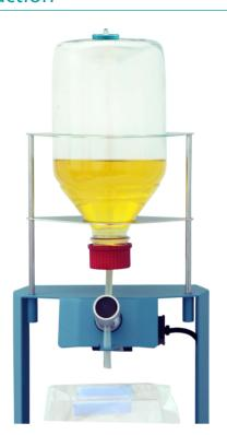
Gravimetric dilutions are automated and simplified by the Pinch Dilutor. The Pinch Dilutor has been specially designed to drive diluents from media containing bottles or ready to use media bags.
