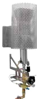
**Exhaust torch** to burn exhaust gases which are generated during the process. The torch is gas heated and will be operated with propane gas. If a catalytic afterburner cannot be used for the process this torch is recommended.
