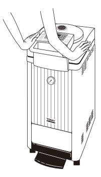
② Select a place which is not subject to direct sunlight and is well ventilated. Install the autoclave with a clearance of 150 mm or more behind the autoclave and 50 mm or more at both sides. Provide sufficient space at the front and above the autoclave.
