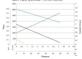
FLOW RATE NOMINAL: 950 mL/min (@ 2.07 Bar) FLOW RATE MAX: 3000 mL/min (@ 0psi, 0 Bar)
