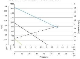
FLOW RATE NOMINAL: 325 mL/min (@ 2.07 Bar) FLOW RATE MAX: 1650 mL/min (@ 0 Bar)
