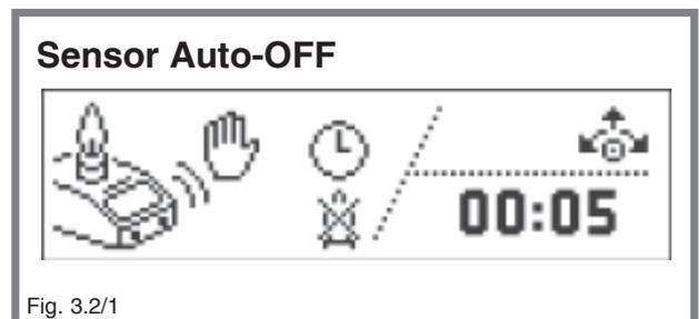
**!** If the **DoubleClick** function is switched off, the flame ignites **IMMEDIATELY** if the IR sensor is activated, i.e.: if a hand or an object is within the detection range!
