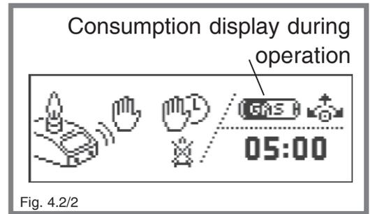
Confirm the type of cartridge by pressing the function knob **(1)**. In the 2nd step the burning time can be individually adjusted to achieve even more precise timing if necessary. By pressing the function knob **(1)** the value set is memorized and the menu item is exited.
