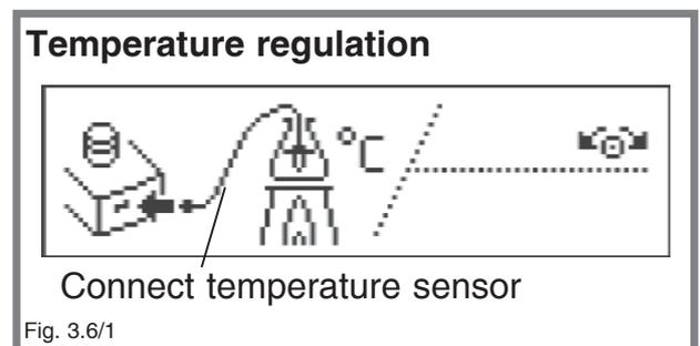
**i** During the temperature regulation program, the timer only starts to count down once the nominal temperature has been reached.
