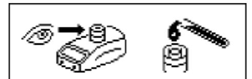
Check burner head (6) for clogging
