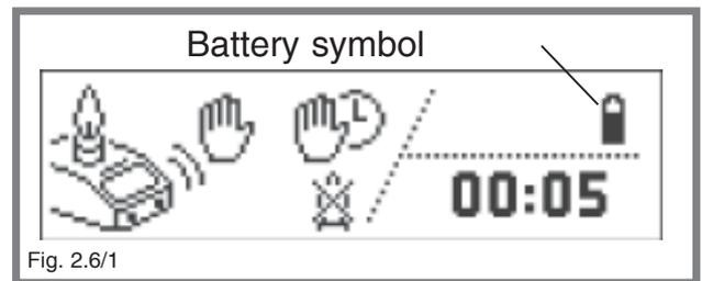
**i** The batteries are charged only if the power cord of the included power supply is inserted directly into the socket (9). If the power supply is connected indirectly over a foot pedal (optional) so that the power cord is inserted in the socket of the foot switch, the batteries are not charged for technical reasons.
