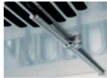
Multi-conductor temperature sensors
