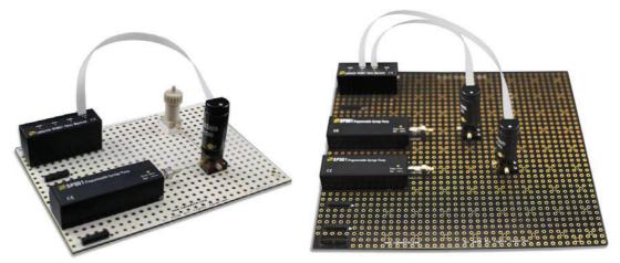
Figure 2. uPB-05 and uPB-08 Breadboards with uDevices.
