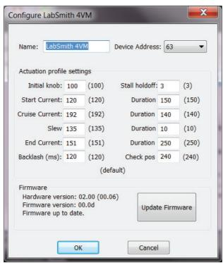
Figure 38. Configure Device Dialog Box for a 4VM01 Valve Manifold.
