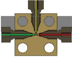
Figure 40 T-Interconnect Showing Properly Installed Capillary (Green), Improperly Seated Capillary (Yellow), and Capillary Not Protruding Through Fitting (Red).
