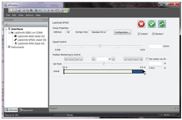
Figure 8. Control Panel for Syringe Pump.
