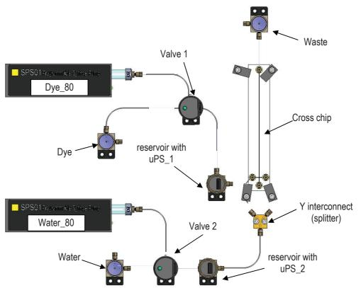
Pressure regulated hydrodynamic flow application (iBB breadboard, 4VM manifold, and 4AM manifold not shown for clarity)
