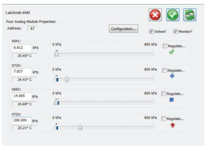
Figure 14 Typical Analog Manifold Control Panel view.
