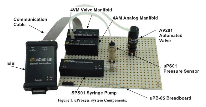
The EIB can also connect directly to a single SPS01 syringe pump, to a 4VM01 valve manifold, or to a 4AM01 analog manifold, without a breadboard.
