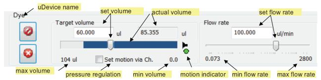
Figure 18 Syringe pump control options in the Device Control Overview Windown
