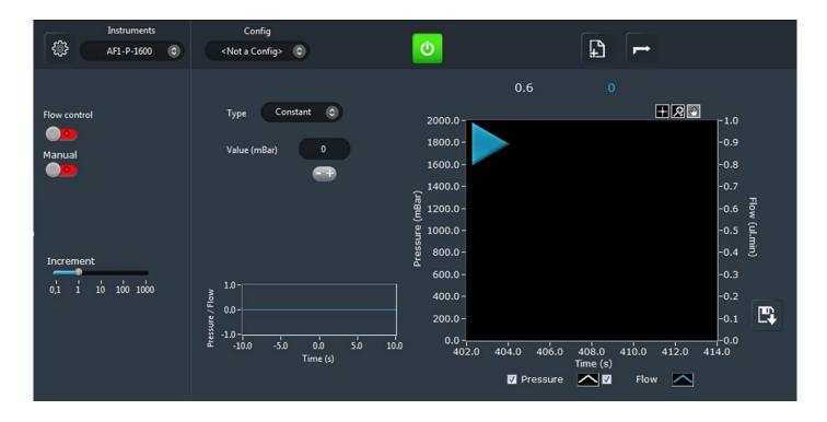
In the main AF1 window you will find information about the current state of your instrument, controls and configurable parameters.
